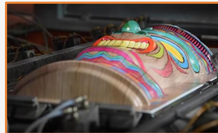
7. Thermoform the printed sample**.
